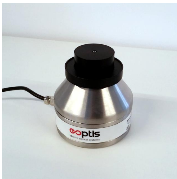
Step 3. Acquisition of White Calibration standard
